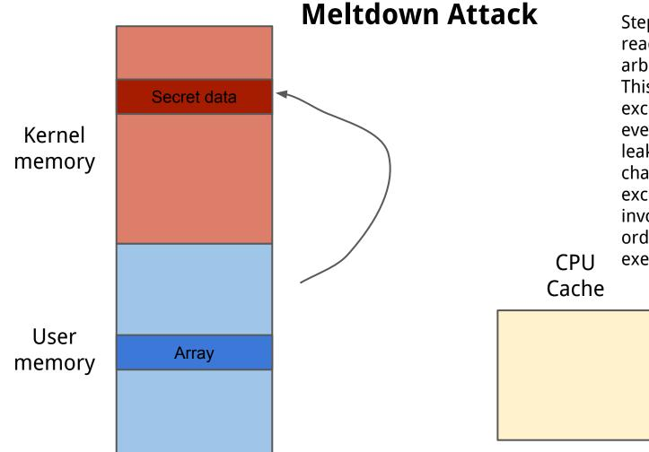
Step 1: A user process reads a byte of arbitrary kernel memory. This should cause an exception (and eventually will), but will leak data to a side channel before the exception handler is invoked due to out of order instruction execution.
