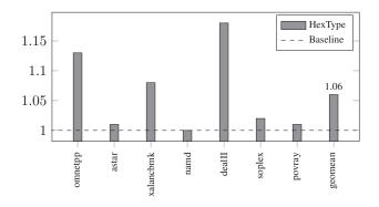
8) Clang CFI: We used the official version of LLVM/-Clang 6.0.0 to compile the baseline binaries, and used the -fsanitize=cfi flag for that same compiler to generate the Clang CFI binaries. Clang CFI inserts checks (i) for casts between C++ class types and (ii) for indirect calls and C++ member function calls (virtual and non-virtual). We enabled -fno-sanitize-trap to print diagnostic information.
